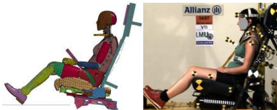
Figure 1.2. EvaRID V1.0 model run in a test set-up to compare its dynamic response to those recorded in volunteer tests run in the same test configuration.
